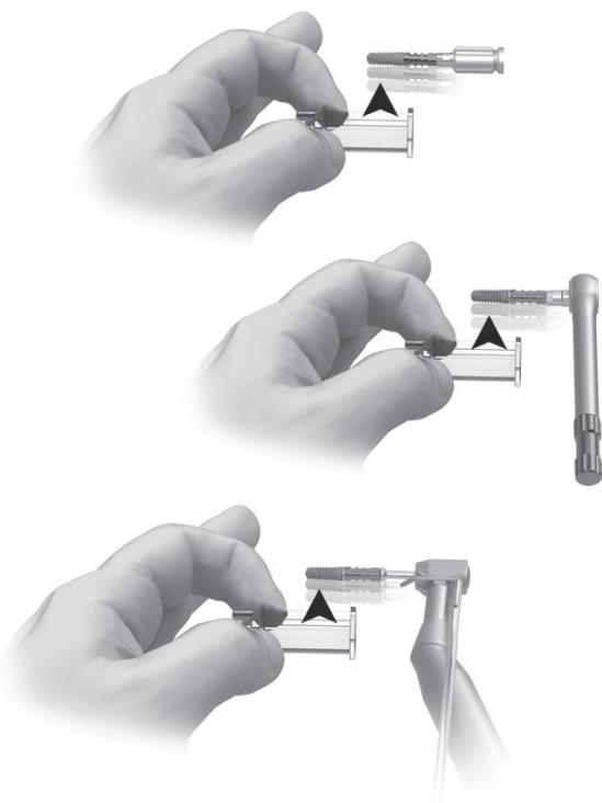
**EN** Remove the implant-ZPlus® Mount assembly by pulling up the vial vertically.
